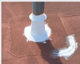
VFI-993 Flashing Grade Silicone is a high build, single component silicone sealant designed to seal abnormal roof penetrations that cannot be covered with standard sprayers or rollers. VFI-993 can be applied by brush, trowel or putty knife and delivers the same protection and waterproofing as Silicone Coatings, *SEALGUARD* VFI-990 SILICONE and *SEALGUARD* VFI-991 SILICONE.
